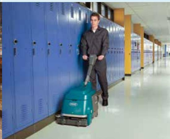
Tennant ec-H2O NanoClean® technology electrically converted water is created by an on-board e-cell that generates millions of very tiny microscopic bubbles known as nanobubbles that promote the cleaning efficacy of the solution. This next generation solution offers the same great benefits of the first generation and now cleans better and cleans more soils in more applications. The name NanoClean, refers to the generation of nano-scale bubbles that are an important part of the cleaning mechanism.
